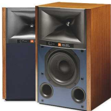
ABOVE: JBL's 4309 sports a compression driver mounted into an HDI horn, see p58
